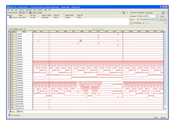
Input pulse bottom, address middle, and difference between stored average and pulse top. Four impurities introduced, with a marker embedded in the code to show where the block repeats.
