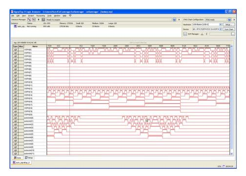
Since, as we have said, the sample points are effectively random, we expect the average to hover around the overall average of the pulse input value, which, including all of the 0's in between, comes out to 20.23 volts. A look at the above figure shows the algorithm's computed average to be around 16volts for any given cell—satisfactory, taking the aforementioned truncation error into account.
