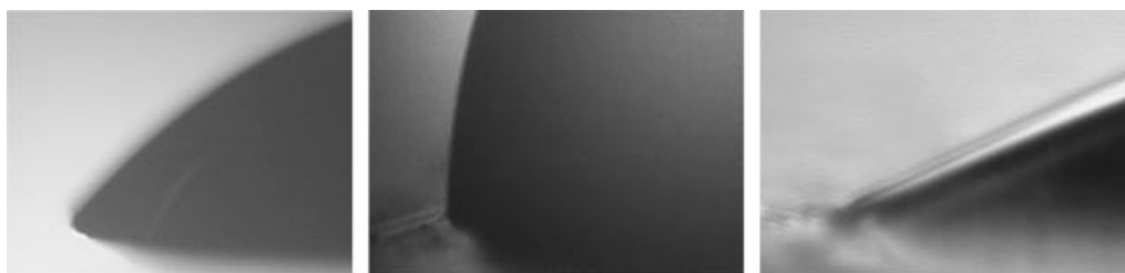
Figure 25. Photographs of the wetting behaviour of water. From left to right: water drop on cleaned glass surface, water drop on flat PPX film surface, water drop on nanostructured PPX film surface (see Figure 22). All contact angles were measured by the sessile drop method.
