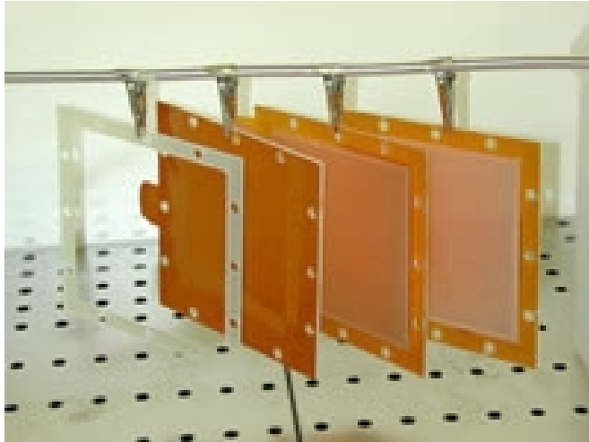
10x10 cm 2 GEM stretched and glued on frames
