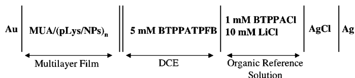
Scheme 3. Schematic illustration of the electrochemical cell and electrolyte compositions.
