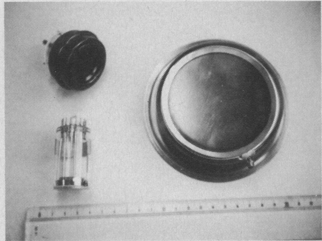
Fig. 1 Some of the custom-made gas photodiodes, having an active photocathode diameter from 19 to 80 mm.
