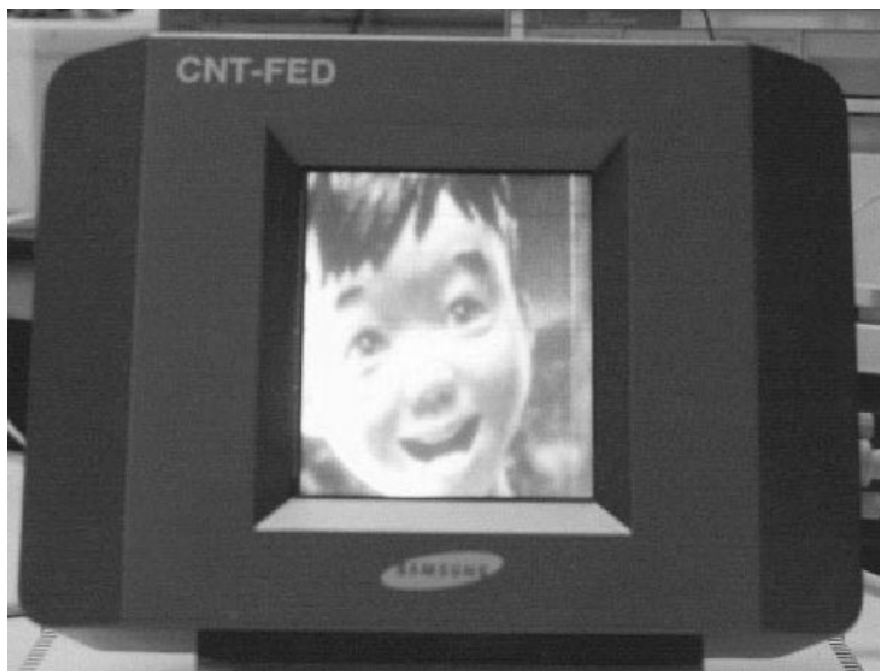
Figure 17. Prototype of a CNT field-emission display (Chung et al. 2002) with a gate structure, an active area of 12.7 cm in diagonal, full colour and 100 Hz.
