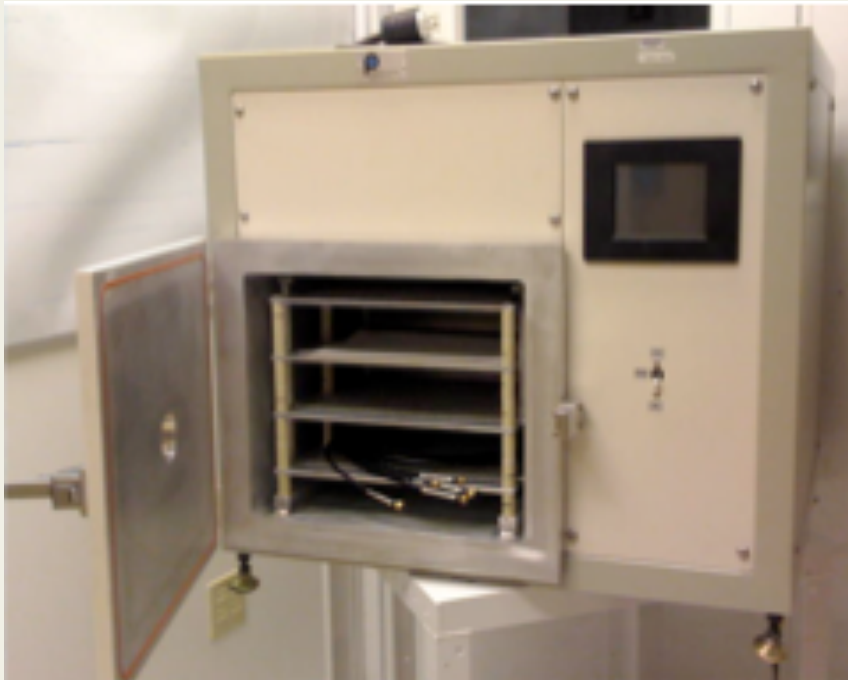
Large plasma asher installed in clean room.
