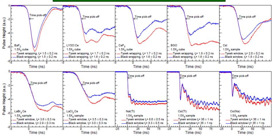
Measured rising time is dominated by photo-detector response, and is affected by light propagation in crystal.
