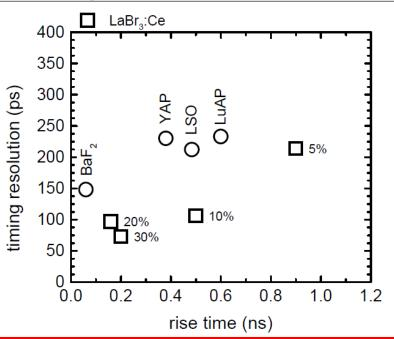
Time resolution achievable: 100 ps for TOF-PET with MCP readout.
