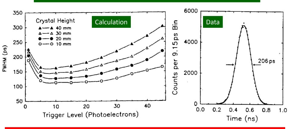
200 ps FWHM, or 60 ps  $\sigma_{\text{single}}$ , measured with BaF<sub>2</sub> & Hamamatsu R3377 PMT readout: a factor of three better than commercial system
