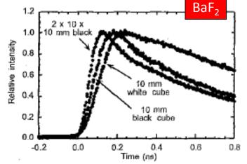
Excitation: 60 ps FWHM x-ray pulse Detector: MCP with 45 ps response
