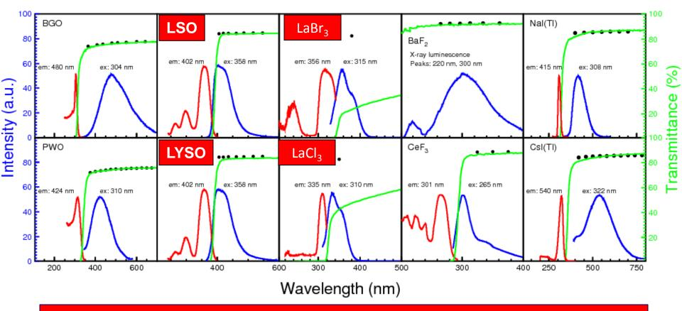
Poor transmittance indicates scattering centers: LaBr<sub>3</sub> and La Cl<sub>3</sub>
