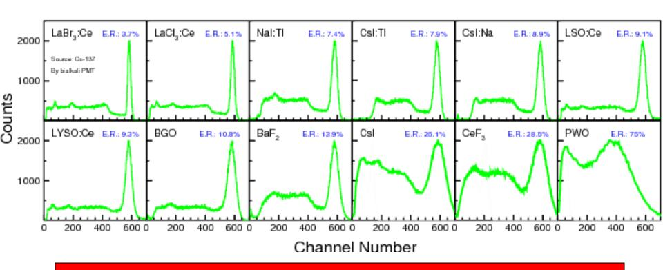
2% resolution and proportionality are important for y-ray spectroscopy between 10 keV to 2 MeV
